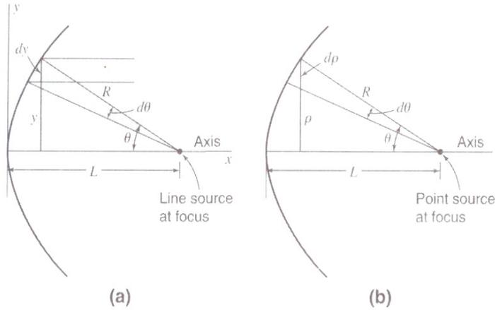
Fig 6.9 : Cross Sections of cylindrical parabola (a) and of paraboloid of revolution (b)
