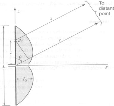
Fig 3.8: Relation for symmetrical thin linear center-fed antenna of length L. Relation for symmetrical thin linear center-fed antenna of length L is as shown in figure 3.8.
