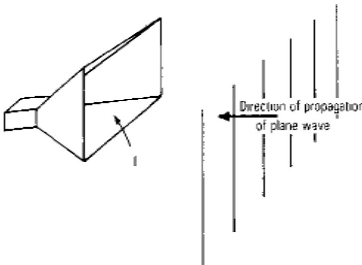
Let the poynting vector or power density of the plane wave be  $S$  watts/sq –m and let the area or physical aperture be  $A_p$  sq-m.If the Horn extracts all the power from the Wave over its entire physical Aperture  $A_p$ , Power absorbed is given by
