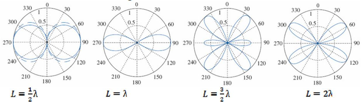
Fig 3.11: The  $E$ -plane radiation patterns for dipoles of different lengths
