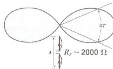
Fig 3.9: (a) Far field pattern of  $\lambda/2$  antenna b) Far field pattern of full wave antenna
