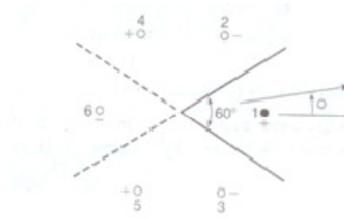
Fig 6.6 : A 60 deg corner reflector with images used in analysis
