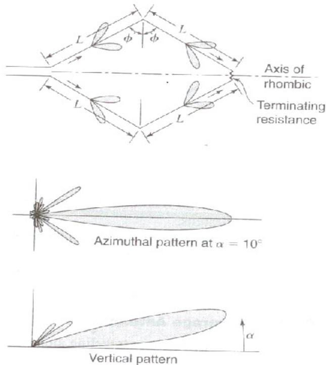
Figure 3.14: Rhombic antenna
