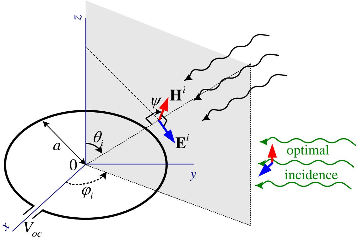
The open-circuit voltage at the loop terminals is induced by the time-varying magnetic flux through the loop:
