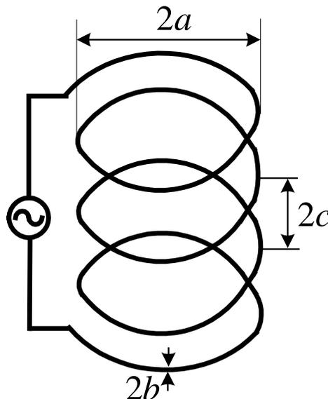
The ratio  $R_p / R_0$  has been calculated for different relative spacings  $c / b$ , for loops with  $2 \leq N \leq 8$  in:
