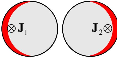
When the spacing between the wound wires is very small, the loss resistance due to the proximity effect might be larger than that due to the skin effect. The following formula is used to calculate exactly the loss resistance of a loop with  $N$  turns, wire radius  $b$ , and loop separation  $2c$ :
