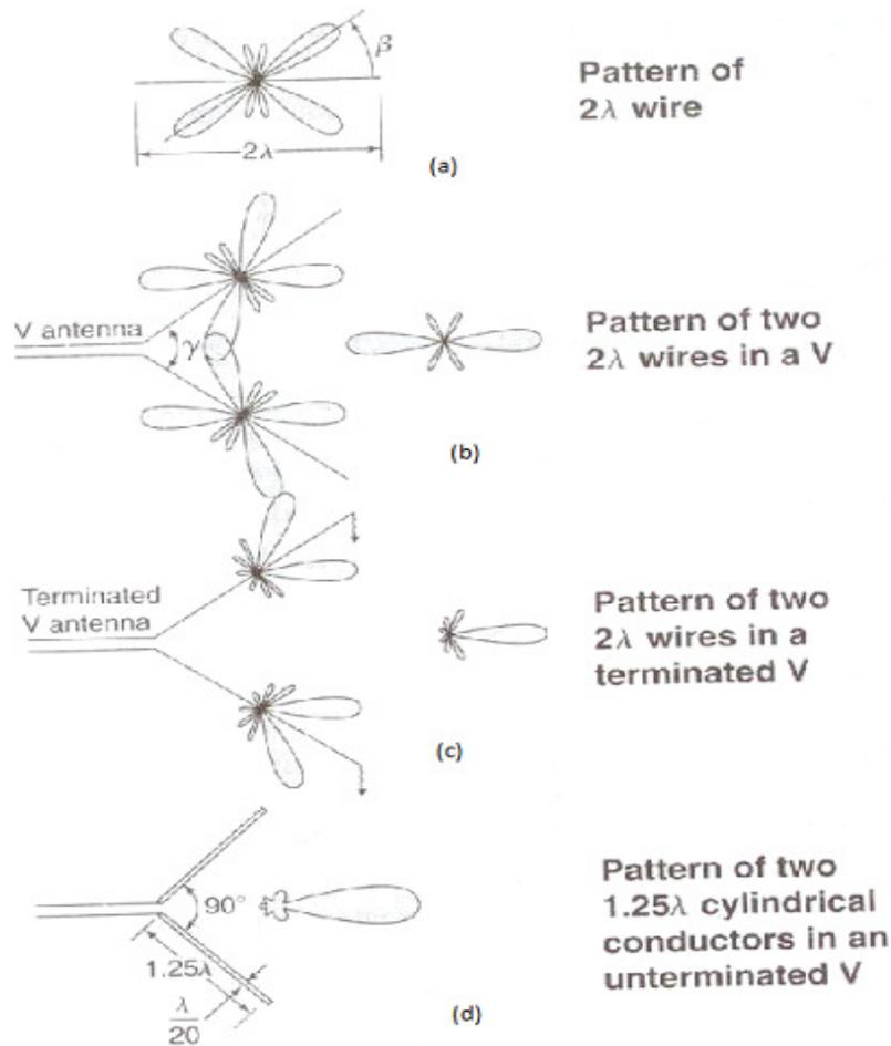
Fig 3.13: a) Calculated pattern of  $2\lambda$  wire with standing wave, (b) v antenna of two such wires, (c) terminated V antenna with legs  $2\lambda$  long and (d) V antenna of cylindrical conductors  $1.25\lambda$  long with measured pattern.
