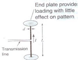
Fig 3.1: A short dipole antenna
