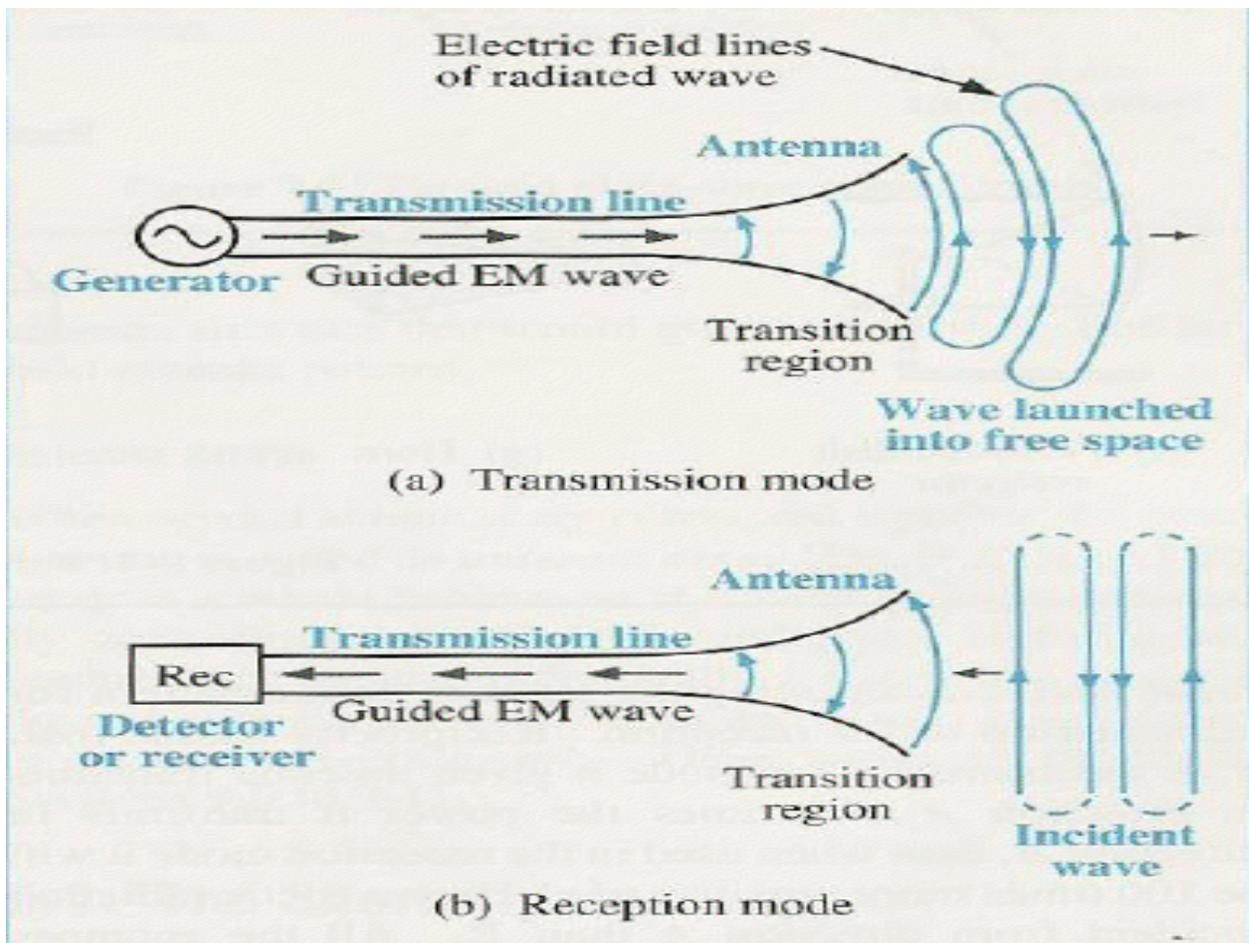
**b) As Receiving Antenna** –Active radiation by other Antenna or Passive radiation from distant objects raises the apparent temperature of  $R_r$ . This has nothing to do with the physical temperature of the antenna itself but is
