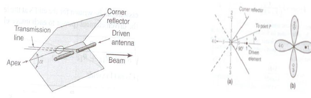
Fig 6.5: Square Corner reflector with images used in the analysis
