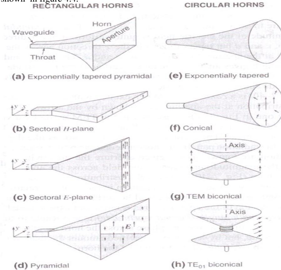
Figure:4.4: Different types of Horn antenna
