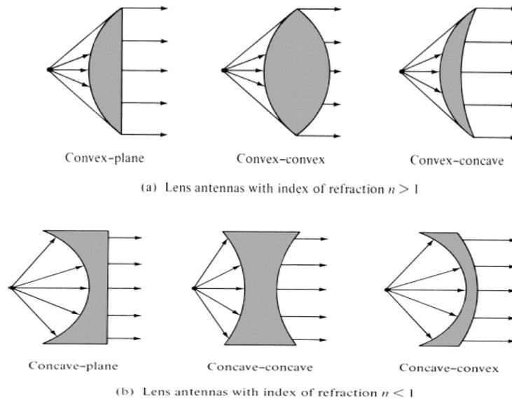
Fig 6.13 : Lens Antenna with different refractive index
