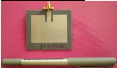
Fig 3.12: Single Microstrip antenna
