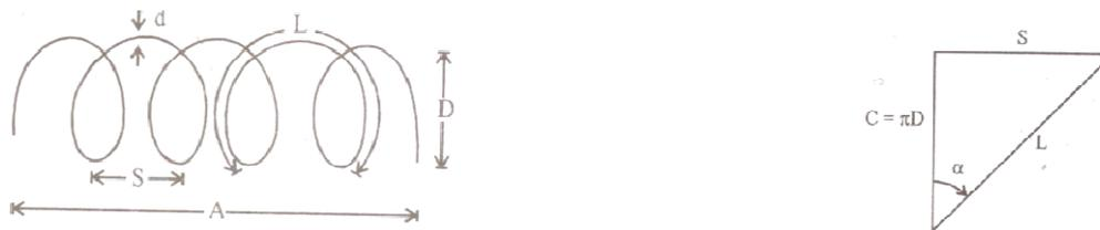
Fig 6.1: Helical Antenna
