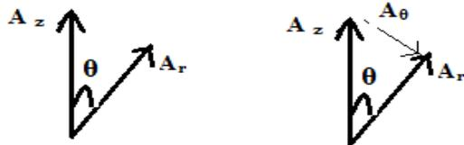
Fig 3.5: resolution of Vector potential into  $A_r$  and  $A_\theta$  components
