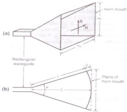
Fig 4.6: Rectangular Horn antenna
