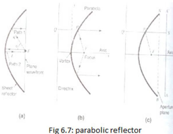
Fig 6.7: parabolic reflector
