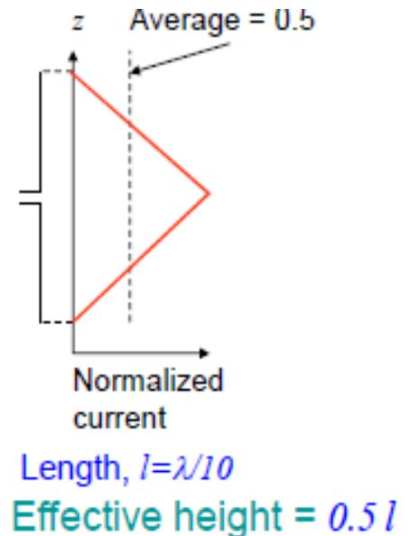
For an antenna of radiation resistance  $R_r$  matched to it's load , power delivered to load is  $P = V^2 / (4R_r)$ , voltage is given by  $V = h_e E$ .
