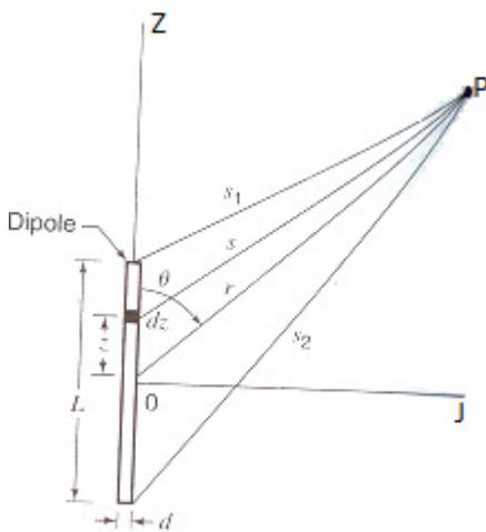
Fig 3.3: Geometry for short dipole
