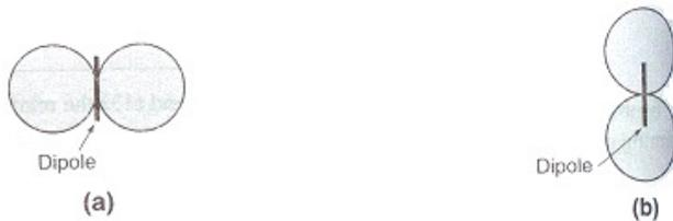
Fig 3.6 (a): Near and far field pattern of  $E_\theta$  and  $H_\phi$  components for short dipole. (b): Near field component,  $E_r$
