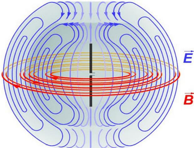
**Fig: Radiation from a dipole**
