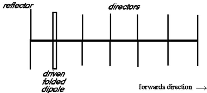
Fig 6.4: Seven segment yagi-uda antenna
