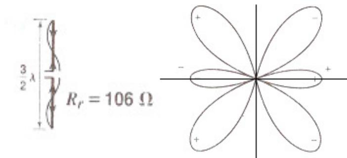
Fig 3.9: Far field pattern of  $L = \frac{3}{2}\lambda$  antenna
