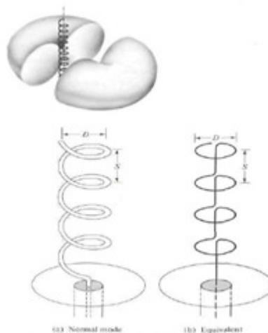
Fig 6.2: Normal mode Helical antenna and its equivalent
