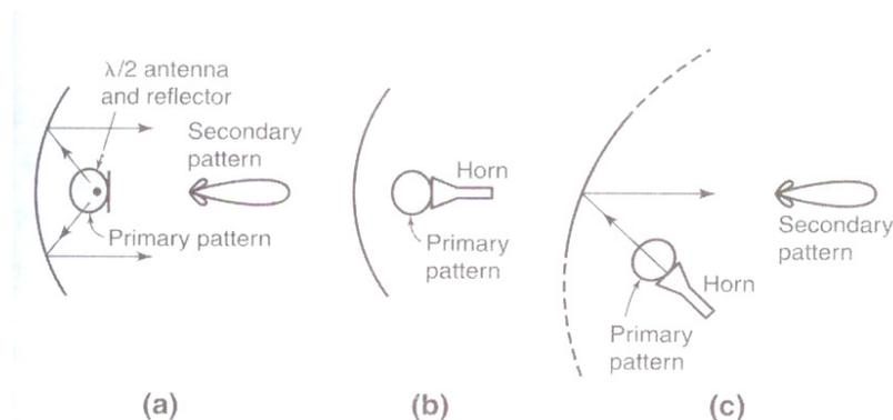
Fig 6.8 : Parabolic reflector with Offset feed
