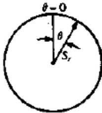
Fig: Power pattern for isotropic source
