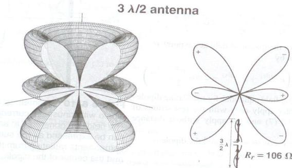
Fig 3.10: Far field pattern of  $L = \frac{3}{2}\lambda$  antenna
