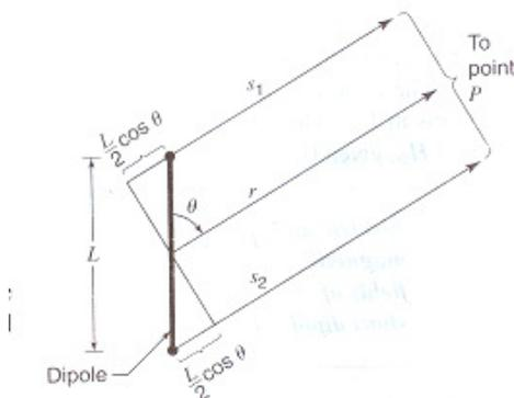
Fig 3.4: Relation for short dipole when  $r \gg L$
