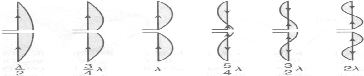
Figure 3.7: Approximate natural current distribution for thin linear center fed antenna of various length.
